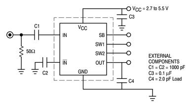
Figure 2. AC Test Circuit
